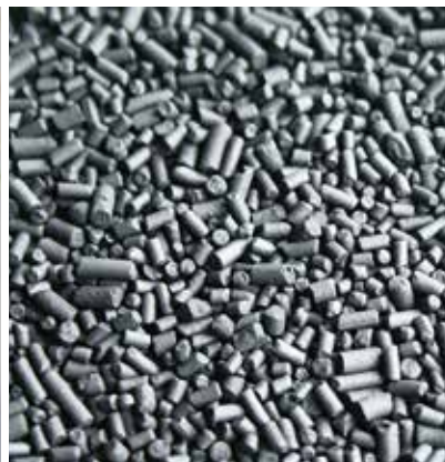
The activated carbon inside the CMS containers binds the oxygen in the atmospheric air, while nitrogen can pass through the containers unhindered.
