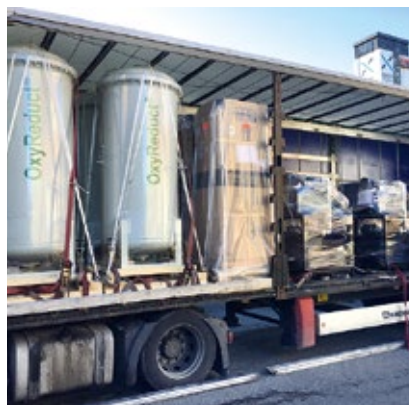
The University of Oslo: an OxyReduct® system with two VPSA-240 nitrogen generators (photo below, prior to installation) protects valuable museum pieces.
